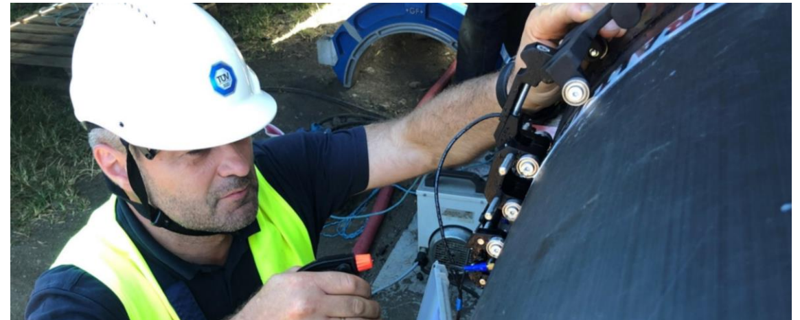
Inspectors in Tahiti use scanners to check the weld beads on pipes:
